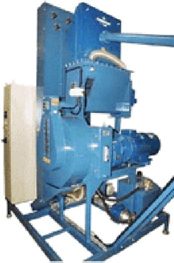
**Fig. 6.13 A 300kg per hour pelleting machine**
