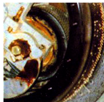
View of Pellet Die and Press Rollers
