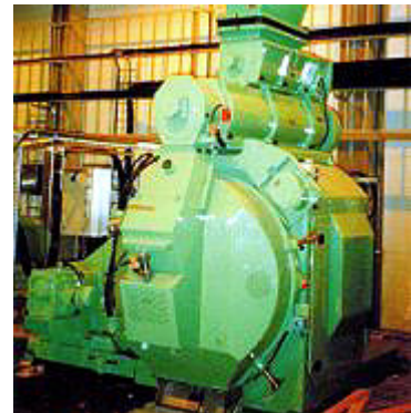
Pellet Press with Conditioning Unit
